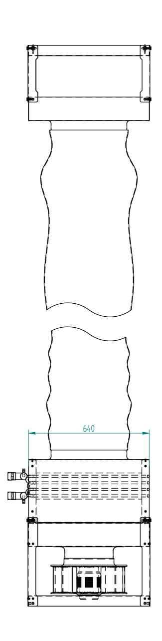
Assembly with coil mounted to fan unit
